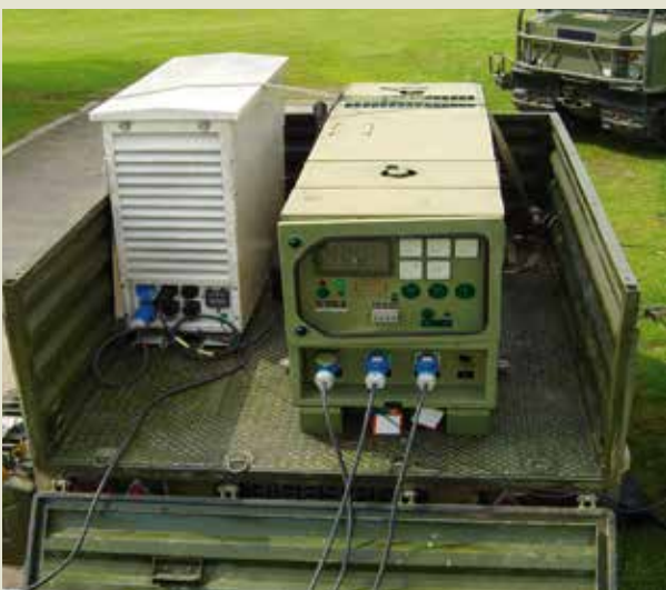
Fully self-contained generator with fuel tank, electrical cabinet. This generator is being used to power a SATCOM unit.
